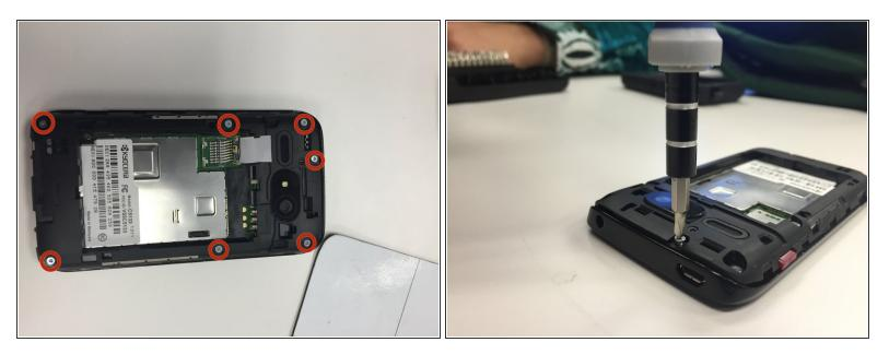
• Remove seven of the 4.9mm tri-head screws. Keep them in a secure location.
