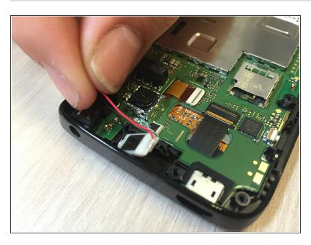
Prior to removing the motherboard, remove the speaker from the top of the device.
