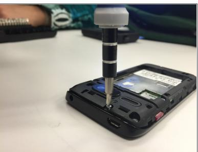
Remove seven of the 4.9mm tri-head screws. Keep them in a secure location.
