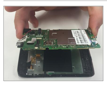
Using fingers, remove the motherboard from its casing.
