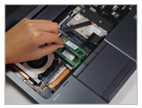
After removing the keyboard, flip the laptop over and remove the other two modules.
