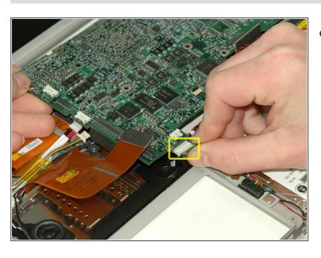
Disconnect the battery cable from the front, left corner of the logic board.
