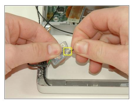
Disconnect the Bluetooth antenna cable from the Bluetooth board.
