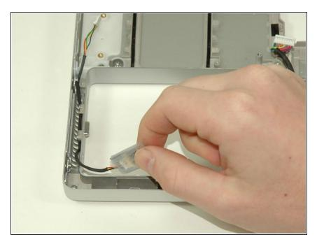
The Bluetooth board and cable should also be free, wedged in the cavity next to the battery compartment. Remove these and set them aside.
