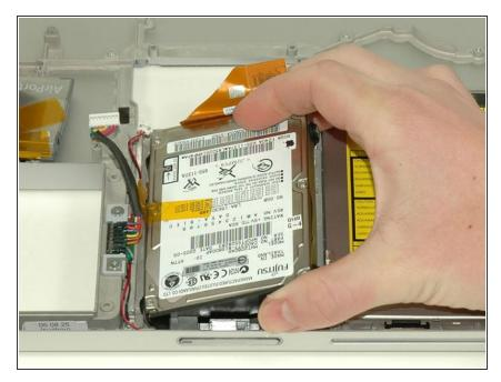
Lift the hard drive up from the right side and remove it from the computer.
