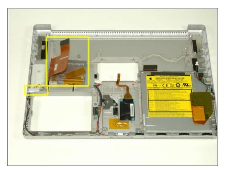
Before going on, remove the loose parts left in the computer. The Airport card and PC card eject button should both be free. Just remove these parts from the computer and set them aside.
