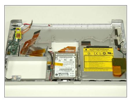
Disconnect the 4-pin power cable and orange ribbon cable from the DC/Sound card.
