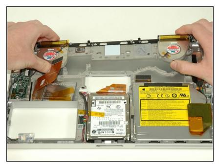
Remove the heat sink from the case, minding the left corner, as it tends to catch in the case (the fans will come out with the heat sink).
