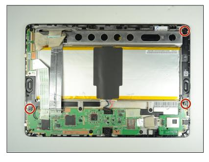
Remove three screws using a Phillips #00 screwdriver.
