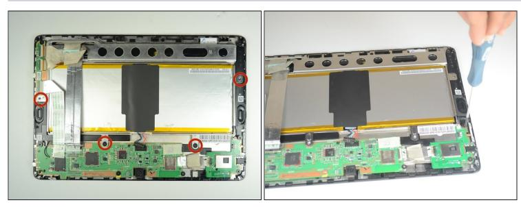
• Remove the four 2 mm Phillips #00 screws holding the battery tray in place.
