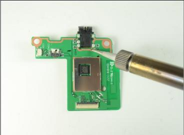
• Using a <u>soldering gun</u>, desolder the headphone jack from the motherboard at each connection to the motherboard.
