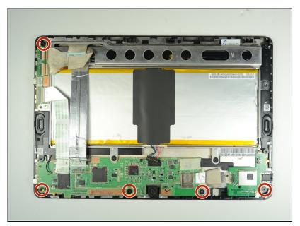
Remove the five screws using a Phillips #00 screwdriver.
