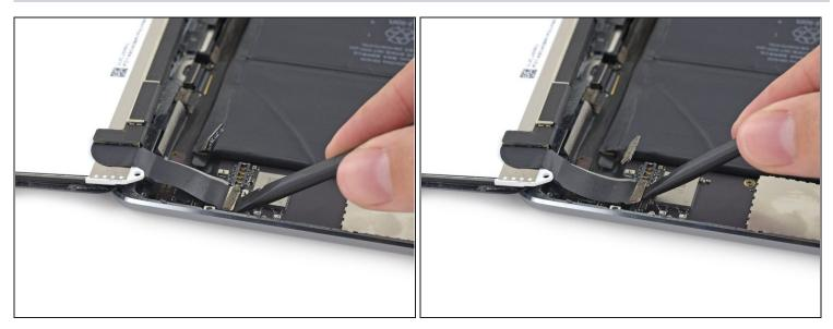
• Use flat end of a spudger to lift the LCD connector up off its socket on the logic board.
