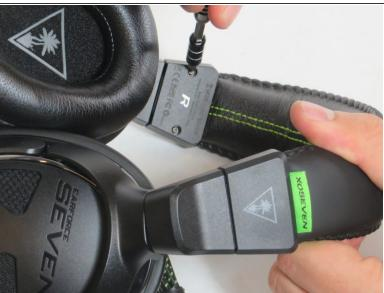
Remove the two 1.0 cmTorx T6 screws using the matching Torx T6 screwdriver.
