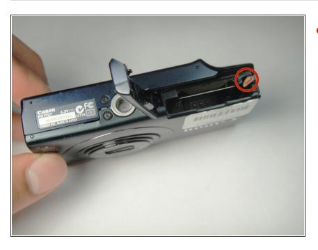
Remove the battery by pushing the orange object outwards; the battery will spring up and out.
