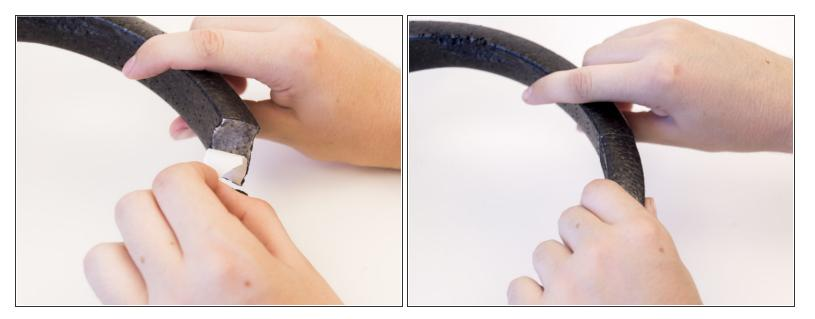
• Peel off the other side of the tape and stick the two sides together.
