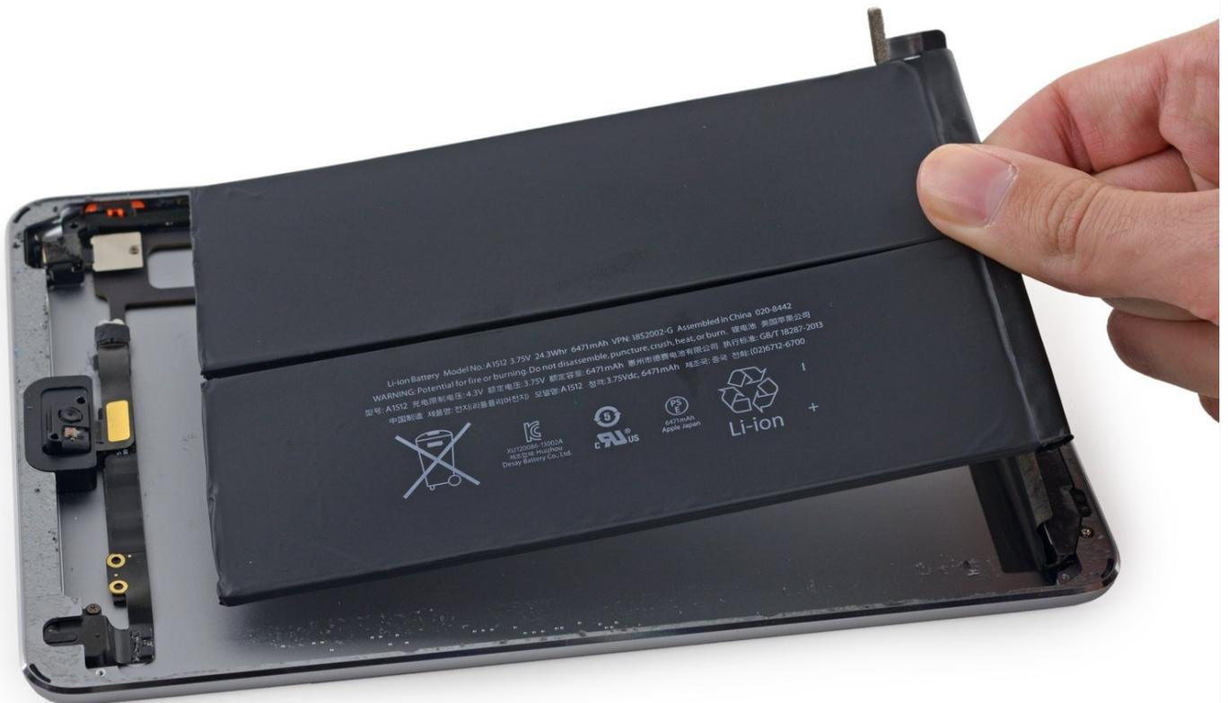
Li-ion Battery Model No.: A1512 3.75V 24.3Whr 6471mAh VPK: 1552002-G Assembled in China 020-8442
