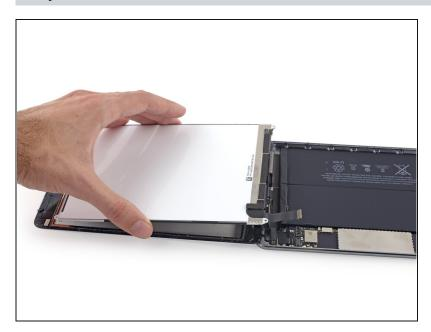
• Lift and remove the LCD from the iPad.
