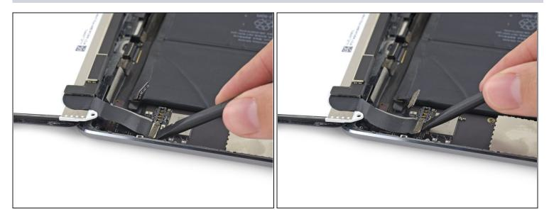
Use flat end of a spudger to lift the LCD connector up off its socket on the logic board.
