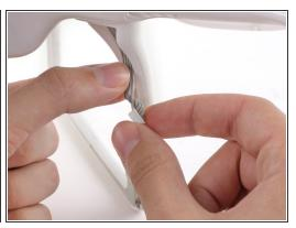
Twist the magnetometer cable as shown to prepare for passing it through the case bottom shell.
