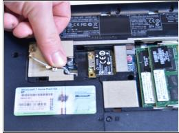
• Use tweezers to disconnect the gray cable and the black cable from the wireless card.
