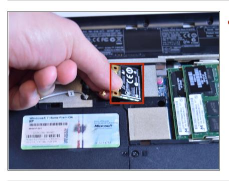
Carefully lift and pull wireless card. It is removed!
