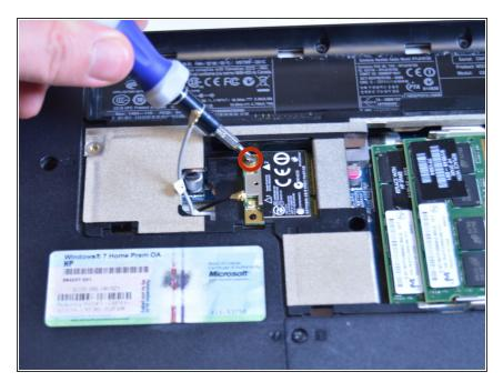
Use a Phillips #0 screwdriver to remove the single 4mm screw from the corner of the wireless card.
