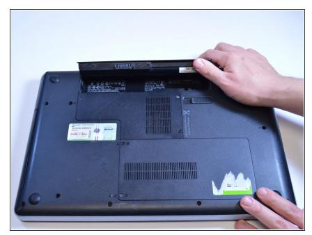
Carefully remove the battery from its compartment.
