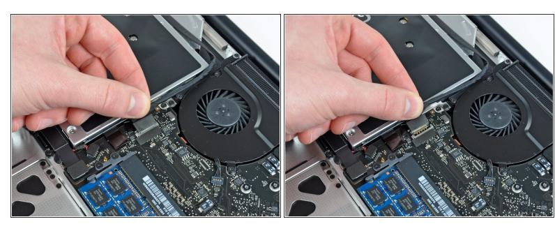
Pull the camera cable away from its socket on the logic board.
