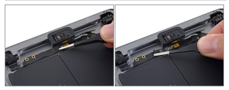
Use a set of tweezers to peel up the small piece of tape covering the microphone cable connector.
