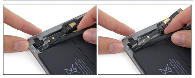
Continue to carefully pry under the cable near the headphone jack.
