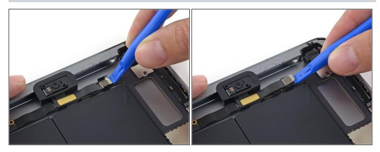
Use a plastic opening tool to lift the front-facing camera cable connector straight up off of its socket on the logic board.
