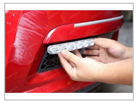
After mounting the bracket, you can lock the LED daytime running light on the bracket.
