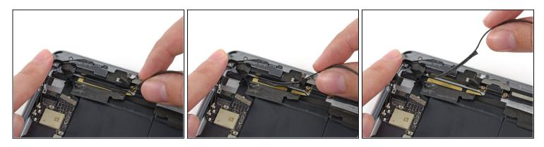
Lift the antenna cable tape up from behind the right speaker.
