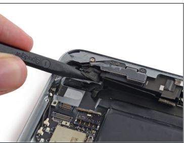
• Use the point of a spudger to lift the antenna cable adhesive up off the rear case.
