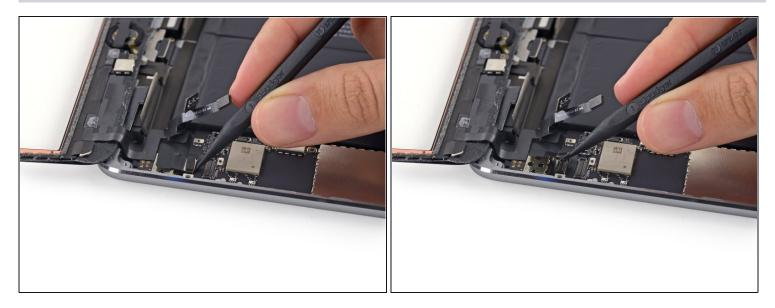
• Use the tip of a spudger to lift the digitizer cable connector straight up off of its socket.
