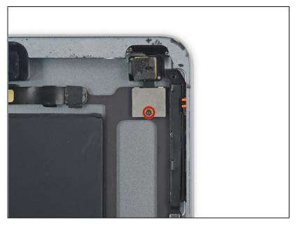
Remove the 1.4 mm Phillips #00 screw securing the rear-facing camera cable bracket.
