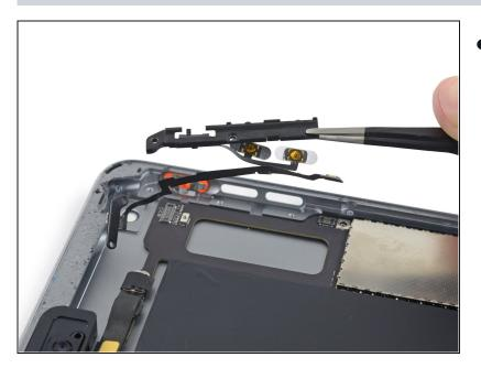
Lift the button assembly carefully out of the rear case.
