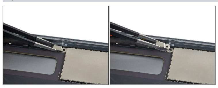
• Remove the case button cable bracket from the iPad.
