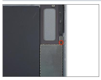
Remove the 1.8 mm Phillips #00 screw securing the case button cable bracket.
