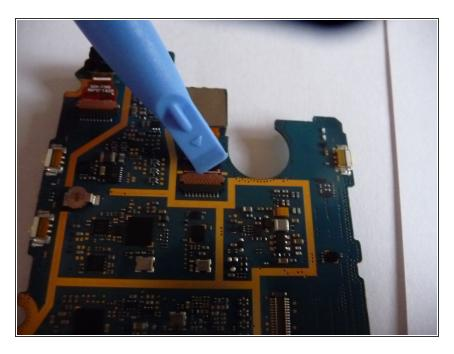
Use a plastic opening tool to disconnect the rear facing camera from the motherboard. To reassemble your device, follow these instructions in reverse order.
