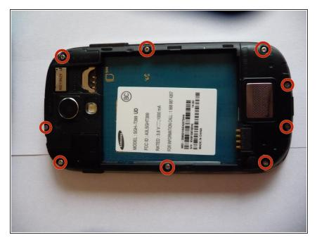
Using a Phillips #0 screwdriver, remove all nine (9) screws attaching the midframe to the front of the device.
