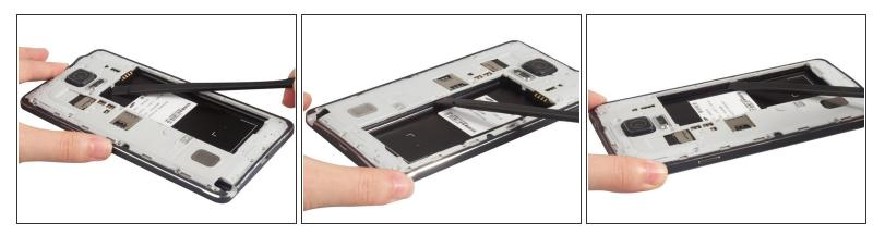
• Loosen the clasp around battery slot.
