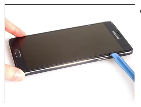
Cut the adhesive sticker along the side of middle housing. Notice: There is no need to separate the LCD screen from mid-plate. So just cut the sticker along side and get the front assembly loosen. Don't do anything else here.
