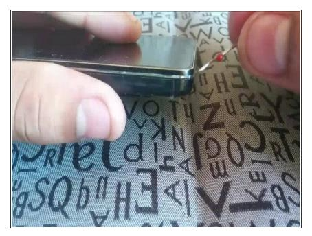
Use an opening pick to pry off the rear case.
