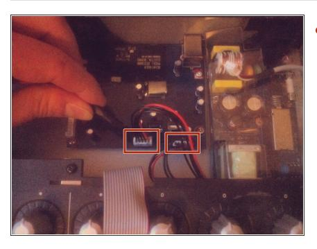
Disconnect the two cables from the lower section to the connector board.
