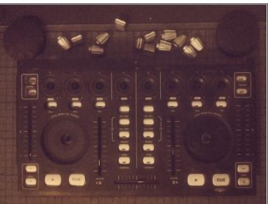
The jog wheels on the front panel can be taken off by using a spudger and levering them out.
