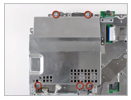
• Remove the five 9 mm Phillips screws securing the power supply to the chassis.
