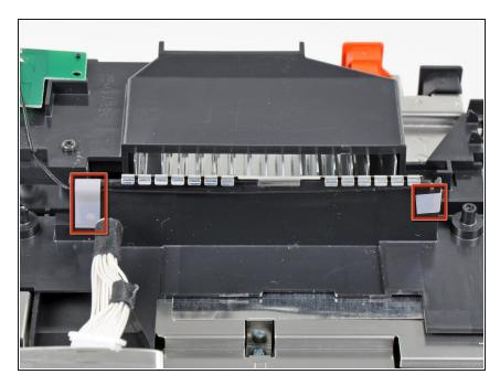
Remove the two pieces of tape securing the second Wi-Fi antenna cable to the plastic bracket near the heat sink.
