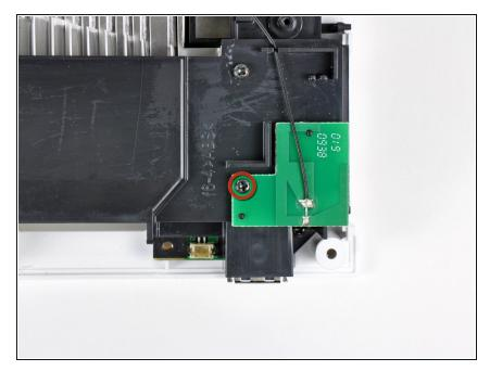
Remove the single 10 mm Phillips screw securing the second Wi-Fi antenna to the top of the fan shroud.
