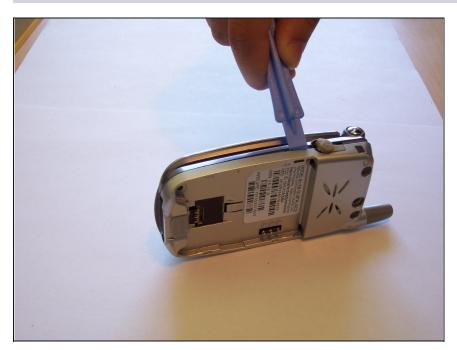
Use a plastic opening tool to separate the front and back casing.
