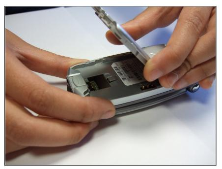
• Lift the battery up from the phone as shown. Replace with a new battery if the old battery has become worn out.
