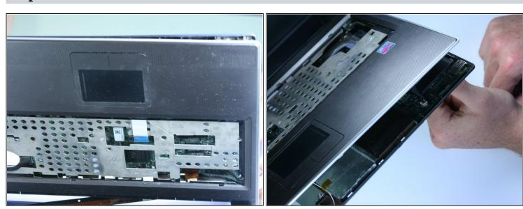
• Use your fingernails or a pry tool to gently separate both halves of the case. Begin at the front and work around the entire case.
