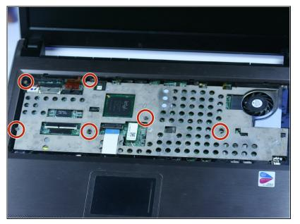
Remove the six screws from below the keyboard with a Phillips #0 screwdriver.
