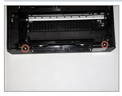
• Use the Phillips #2 screwdriver to remove the two 14.1 mm screws holding the panel in place.
