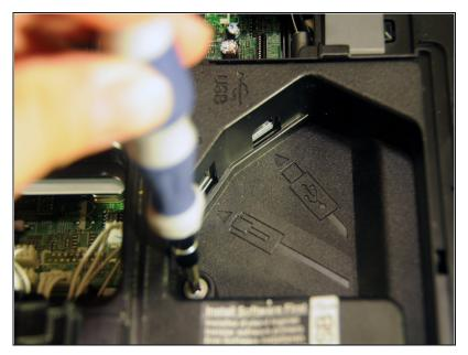
• Use the Phillips #2 screwdriver to remove the 8 mm screw at the center of the device.
