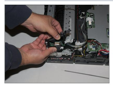
• Squeeze the ends of the cover, then release the cover, revealing the processor unit.
