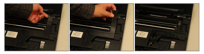
• From the back of the device, use the exposed portion of the panel to begin to lift the panel away from the device.
