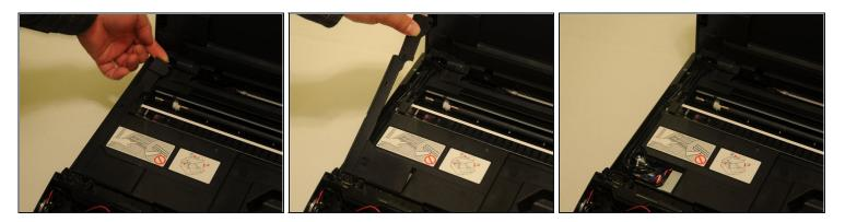
(i) While it is not necessary to use a prying tool, using one may make it easier to lift the panels.
