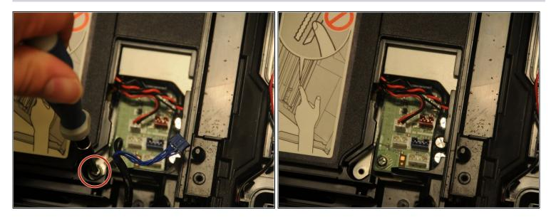
• Use a Phillips #2 screwdriver to remove the 12.1 mm screw to remove the ground wire.
