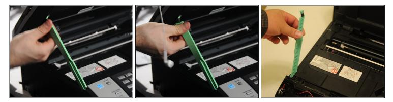
(i) Before removing the unit, apply 2 or 3 pieces of tape to secure the top and bottom of the unit.
