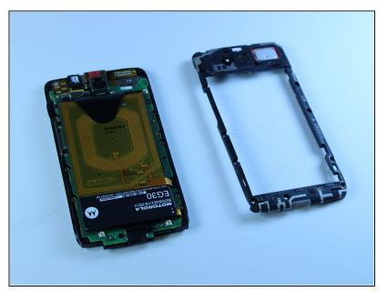
• Carefully separate the housing frame from the motherboard.
