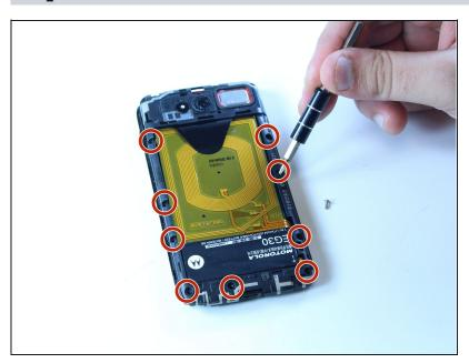
Use a T5 Torx screwdriver to unscrew the nine silver screws from the housing frame.
