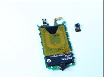
• Use tweezers to remove the camera from the motherboard.
