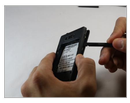
With the spudger, go around the seam of the phone and pry away the back chassis.
