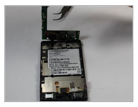
Lift up the motherboard out of the device,
