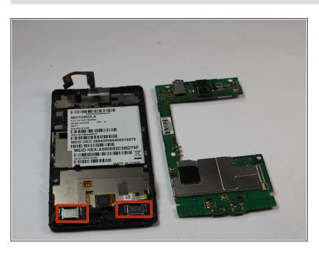
Pry the speakers out using the plastic spudger.
