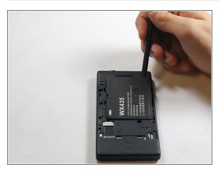
Gently pry out the battery using the spudger
