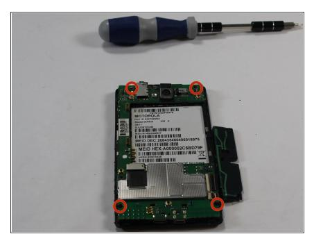
Using the T5 screwdriver, remove all the four screws shown in the picture.
