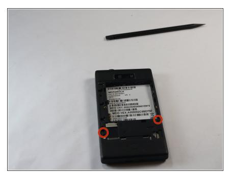
After removing the Battery remove the two screws with a T4 screwdriver.
