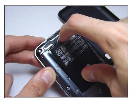
• Lift the battery out of the phone and replace with your new one.
