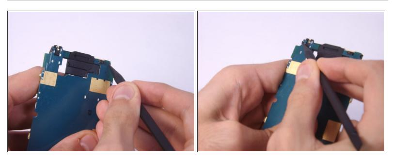
Using the spudger, push the black tabs on the sides of the motherboard off carefully.
