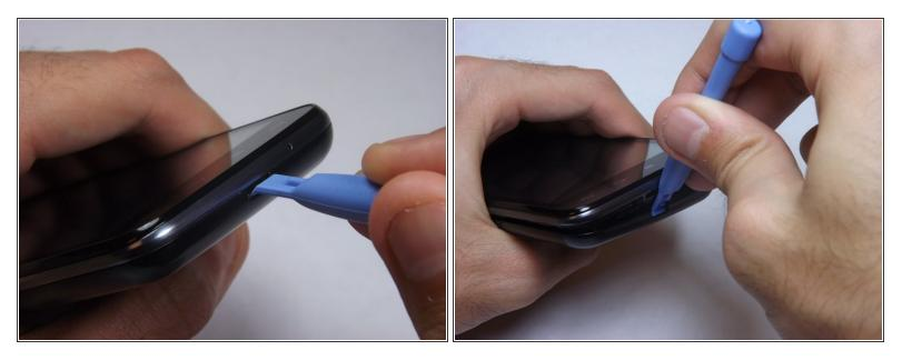
Make sure not to push the tool into the USB port. Doing so may cause damage to your phone.
