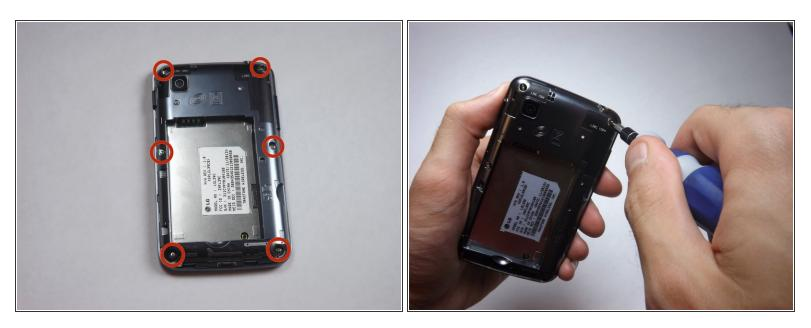
• Use the PH #000 screwdriver to remove the six screws from the midframe
