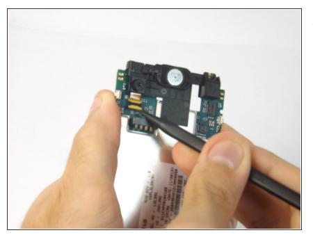
Turn the phone over and pull up the orange tab connected to the camera.
