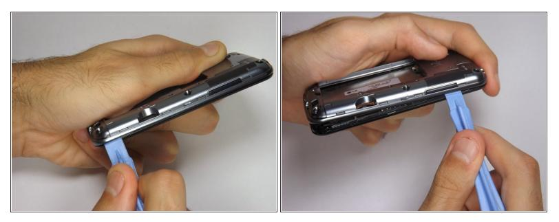
Using the plastic opening tool, work gently to go around the perimeter of the phone and remove the midframe.
