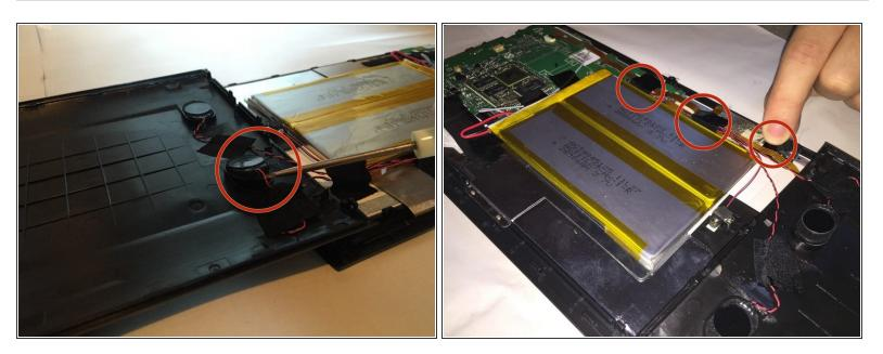
Using a prying tool lift the edge of the speakers where the wires are attached. Follow the wires
