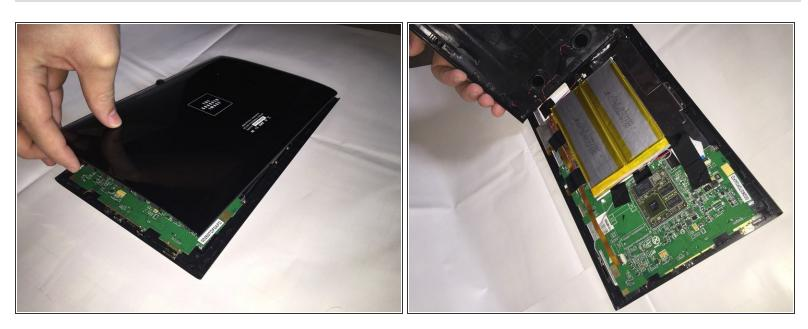
Snap the back cover of the tablet off of the front cover, hence removing the tablet's outer casing.
