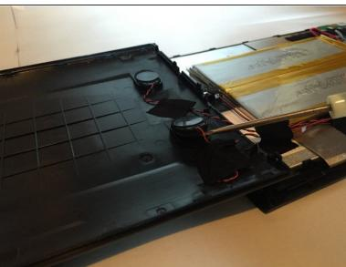
Using the wire snippers, cut the defective speaker wires as close to the circuit board as possible.
