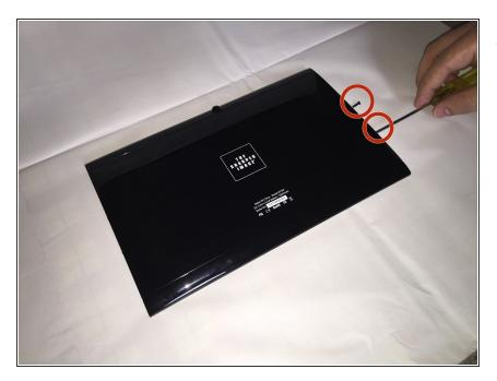
Remove 9 screws by unscrewing the ones behind the panels with a bit driver. There are four screws on one side and five on the other. All which need to be removed.
