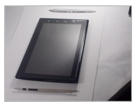
Remove silver side panels with prying tool by snapping them of the outer casing of the tablet.
