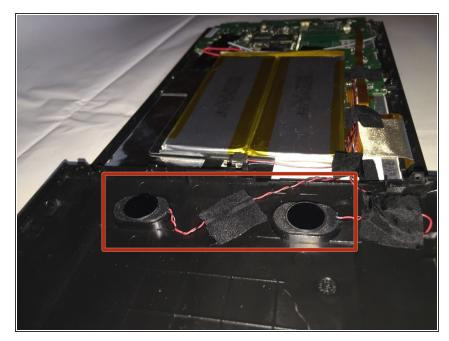
The speakers are located on the inside of the back casing. They are two small black ovals thats are connected with two sets of black and red wires and connect to the logic board.
