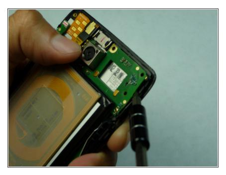
Start by lifting the motherboard using a prying plastic tool like the spudger for example.
