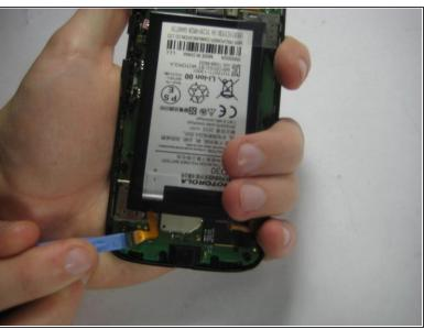
Disconnect the connection between the Battery and the Mother Board by using the Pry tool.
