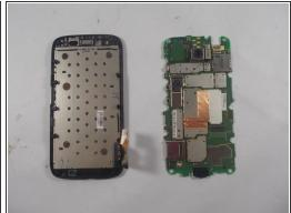
Use the plastic prying tool and slowly work around the edges of the phone to detach the screen from the motherboard.
