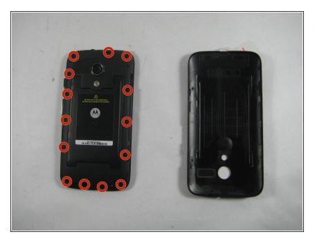
Unscrew the 3.5mm screws, total of 14, located on the back protective cover by using a T5 Torx screwdriver.
