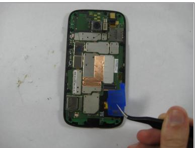
Remove the plastic protective cover by using the tweezers.
