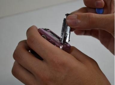
• With a plastic opening tool, gently lift and remove the silver piece on the right side of the camera.
