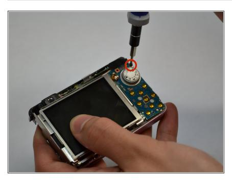
Remove the screw located above the mode dial.
