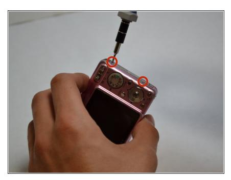
Unscrew the screws on the right side of the camera.
