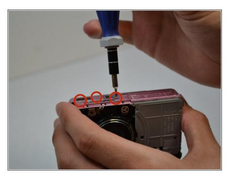
Unscrew the three screws on the bottom of the camera.
