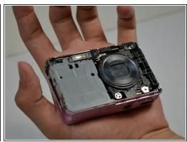
Use a plastic opening tool to carefully lift and remove the front case.
