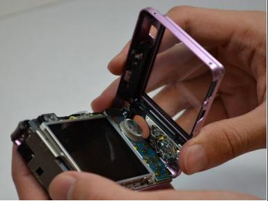
• Use a plastic opening tool to lift and remove the back case.
