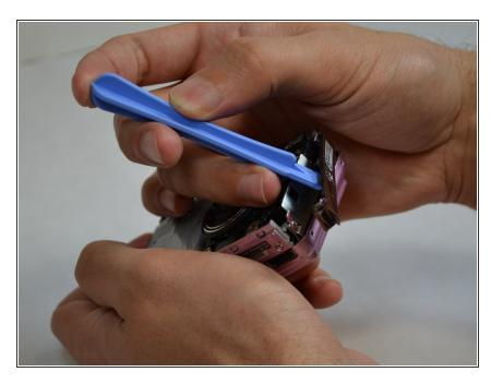
Gently pry the silver piece on the left side of the camera off with a plastic opening tool.
