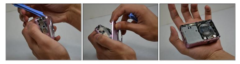
• Use a plastic opening tool to separate the front case of the camera, and gently remove it.
