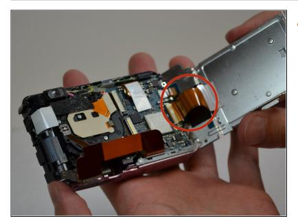
Lift the display from the rest of the camera and gently separate the connecting tape using tweezers.
