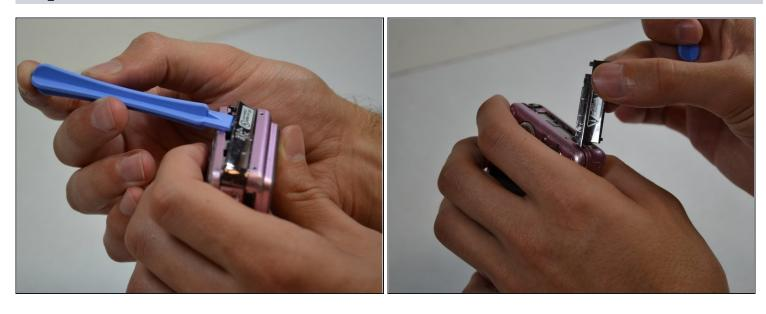
• Using a plastic opening tool, gently lift the side of the silver piece on the right side of the camera until it can be removed.
