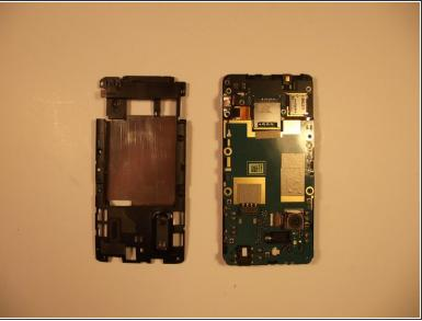
Remove the rear housing by prying around the edge with your Safety Pry Tool
