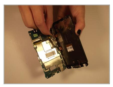
Disconnect the two aluminum flex cables
