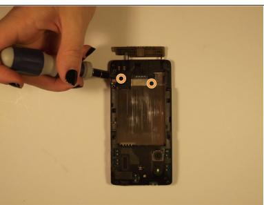
Remove the two revealed screws on the outside (Torx = red, Phillips = orange), and then remove
