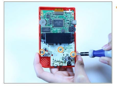
Use a Phillips #1 screwdriver to remove the three screws from the motherboard.
