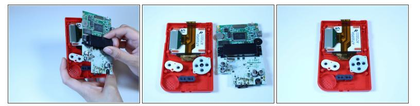
Grab the black piece protruding from the motherboard, and lift up to remove the motherboard.
