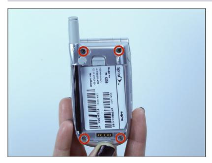
Unscrew all four, 5mm Tri-Wing screws.
