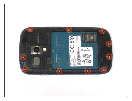
Use the Phillips #000 Screwdriver to remove the 10, 4mm screws holding the plastic frame in place.
