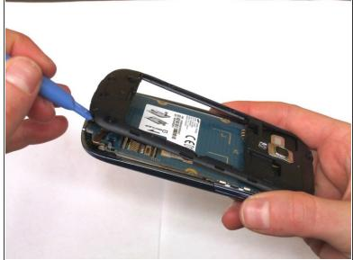
• Using an opening tool, gently separate the plastic framing from the phone.
