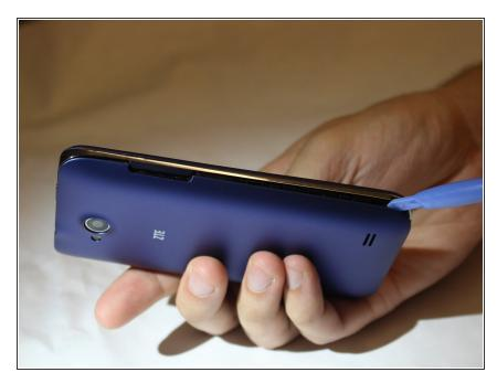
Using your fingernails or a spudger, remove the back panel of the phone.
