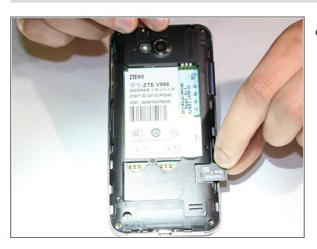
Take the new SD card and insert it into the slot.
