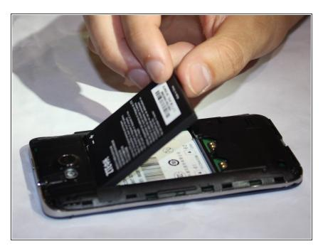
Take the new battery and place it into the slot. The phone should operate normally.
