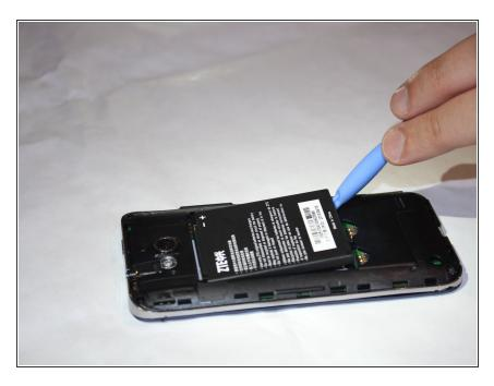
Carefully remove the battery with a spudger.
