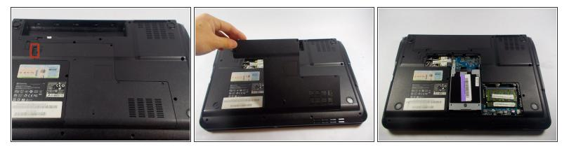
• Place fingers under back plate via the indentation and lift upwards to remove.
