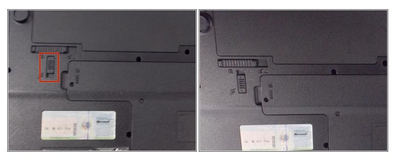
Slide the short slider one towards the unlocked lock symbol.
