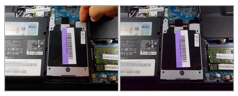
• Grip onto the cover and slide it away from the connector to release the cover and hard drive.
