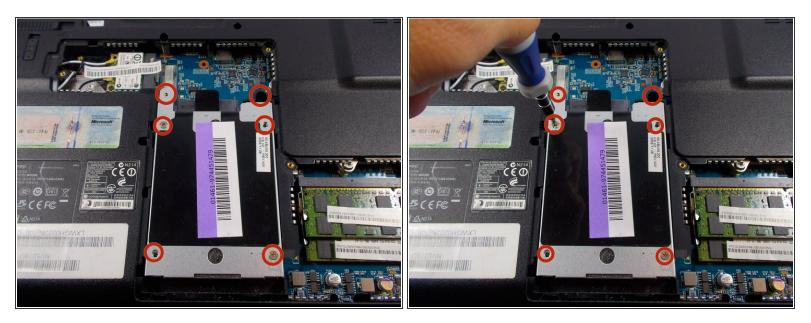
Unscrew the six screws holding the hard drive cover in place
