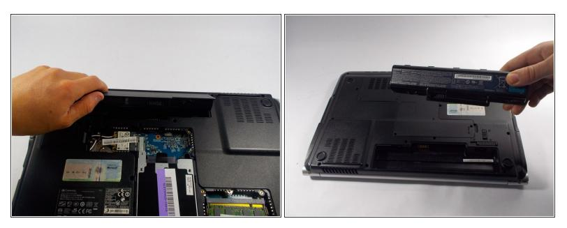
• Grasp the battery's raised end and lift upwards.
