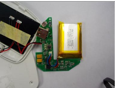
Move the battery slightly, the motherboard can now be lifted from the device case.
