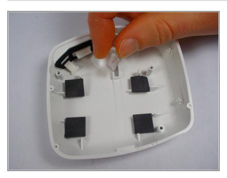
On the device case, beneath the motherboard, remove the power button.
