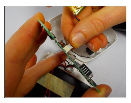
On the underside of the motherboard, remove the battery lead from its connecting terminal.
