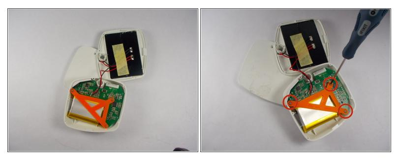
Use a philips screwdriver to remove the three screws securing the battery cradle to the device case.
