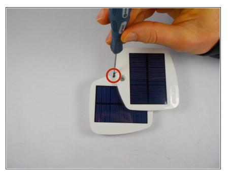
Open the solar panel of the Solio Bolt. Using a philips screwdriver, remove the screw.
