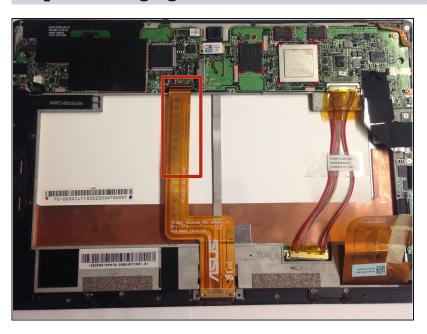
With the battery removed, the charging strip is freely accessible with tweezers.
