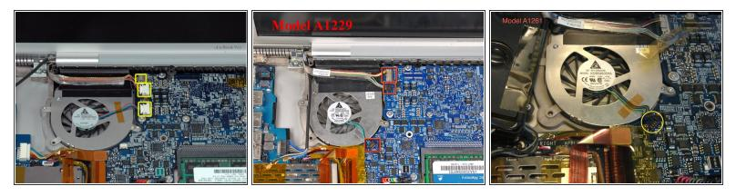
• Disconnect the iSight, inverter, and left fan cables from the left side of the logic board.
