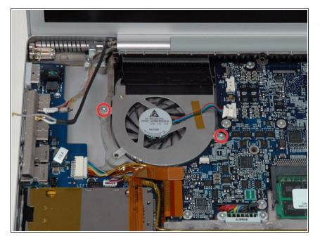
Remove the two silver T6 Torx screws securing the left fan to the lower case.
