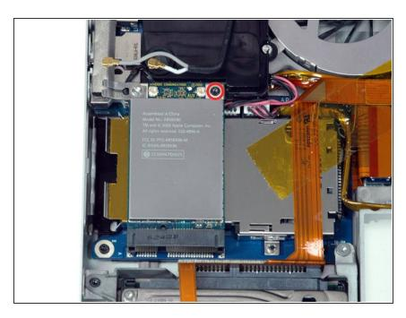
Remove the single black T6 Torx screw from the top right corner of the AirPort Extreme card.
