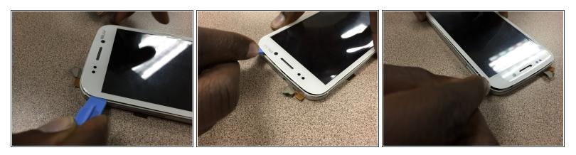
• Once the screen has been heated and the glue is tacky, put a plastic opening tool between the glass screen and the frame. Start lifting the glass away around the whole frame.
