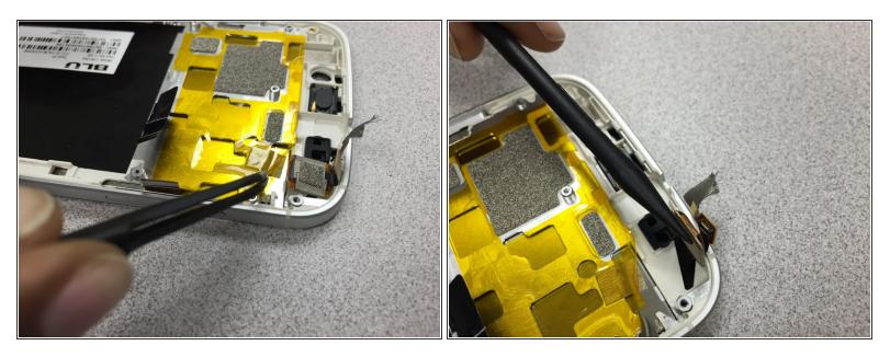
• Using your tweezers, peel back the yellow film to free the cable from the screen.
