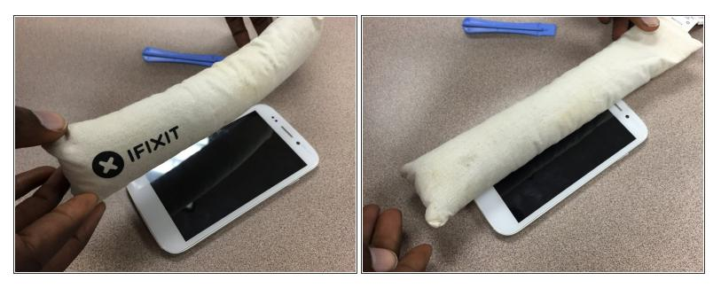
• We used the iOpener tool, heated it up, and placed it on top of the phone for a few seconds to loosen up the glue.
