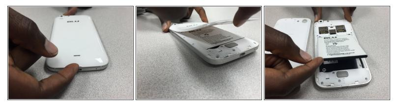
Remove the cover by lifting the notch towards the bottom of the phone. Use your fingernail to lift it up.
