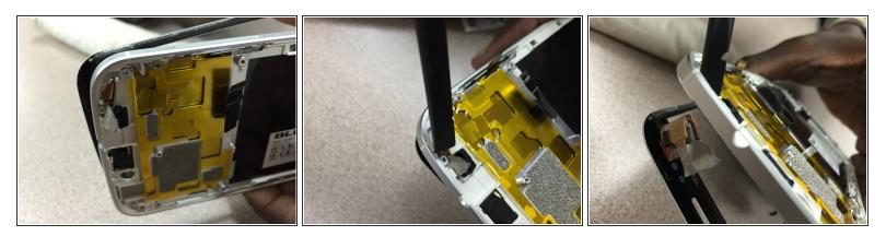
• Take a spudger and gently push the cable through the cutout on the frame to separate the glass.
