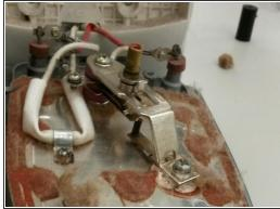
• First remove all the large screws that detach the silver hot plate from the plastic piece attached to it. Lift the white plastic piece to reveal the inner workings of the iron (see last photo attached)
