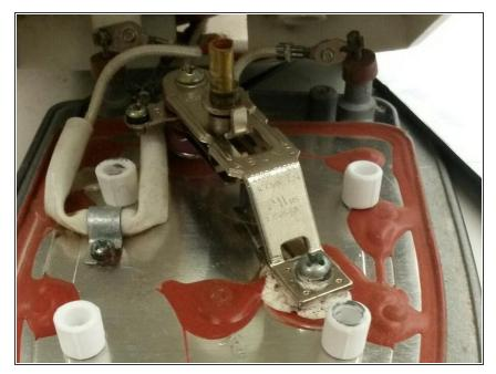
This iron was particularly dusty, clear the dust away with a toothbrush or other small brush. The result is shown in the photo; a clean, dust free iron.
