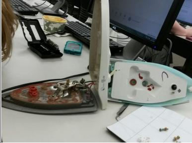
• Remove the smaller screws located near the square(back) end of the iron releasing cords and wires. Also remove little orange rubber gaskets, and white plastic spacers, taking note where everything was. At this point, your iron should be completely disassembled, and should look like the last photo attached.
