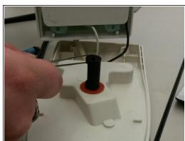
Beginning with the spacers and gaskets, replace these parts where they belong. Then re-install the small internal screws, taking care to reattach the wires and cords with them. Close the white plastic plate onto the metal hot plate and re-attach the larger main screws. Place black dial receptacle into orange slot (as pictured).
