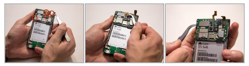
• Use a plastic spudger or your fingers to gently pry up the four flex cables from the main board.
