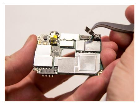
Using the small pliers, disconnect the front camera's flex cable from the main board.
