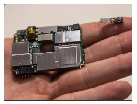
Once the flex cable is disconnected, completely remove the front camera off the main board.
