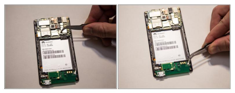
• Lift gently at each connector of the white wire to disconnect the antenna from the port.
